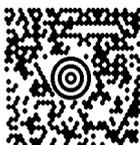
**MaxiCode** is a fixed-size code that holds up to 93 data characters. The symbol is composed of a central bulls-eye locator and offset rows of hexagonal elements. Created by United Parcel Service (UPS), the MaxiCode symbol was designed for quick automated scanning of packages on high-speed conveyor lines (special cameras can read a MaxiCode on a carton travelling at up to 500 feet per minute).
